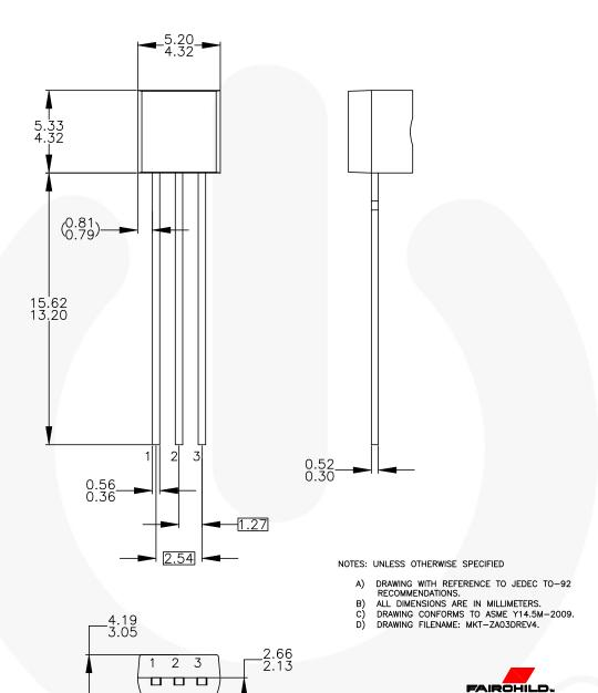
Figure 1. 3-Lead, TO-92, JEDEC TO-92 Compliant Straight Lead Configuration, Bulk Type
