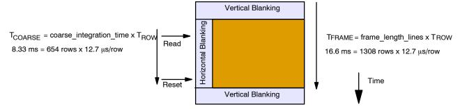
Figure 21. Example of 8.33 ms Integration in 16.6 ms Frame
