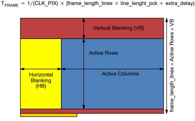
Figure 29. Frame Period Measured in Clocks
