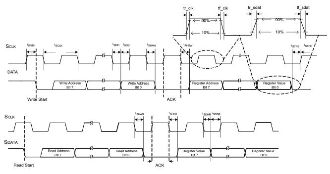
Figure 7. Two-Wire Serial Bus Timing Parameter
