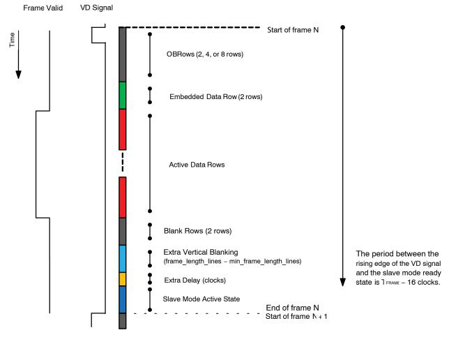
Figure 30. Slave Mode Active State and Vertical Blanking
