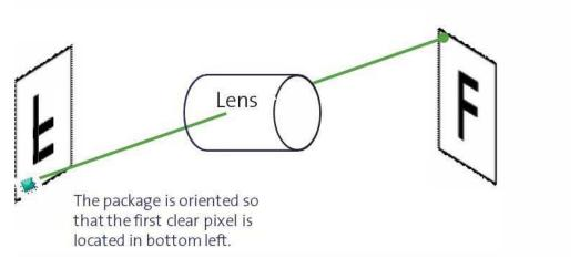
Figure 40. Image Orientation With Relation To Camera Lens
