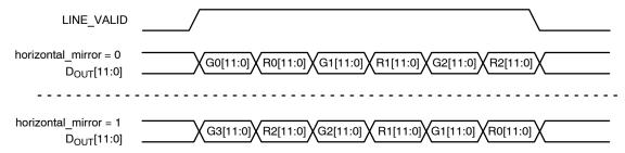
Figure 25. Effect of Horizontal Mirror on Readout Order
