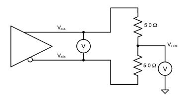
Figure 10. DC Test Circuit
