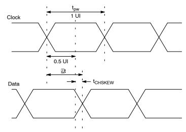
Figure 11. Clock-to-Data Skew Timing Diagram
