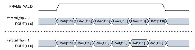
Figure 26. Effect of Vertical Flip on Readout Order
