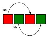
Figure 27. Horizontal Binning in the AR0330CS Sensor
