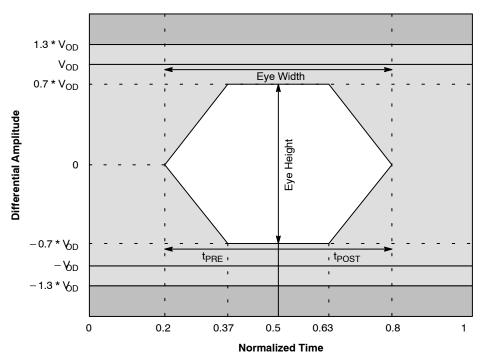
Figure 13. Transmitter Eye Mask
