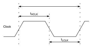
Figure 14. Clock Duty Cycle
