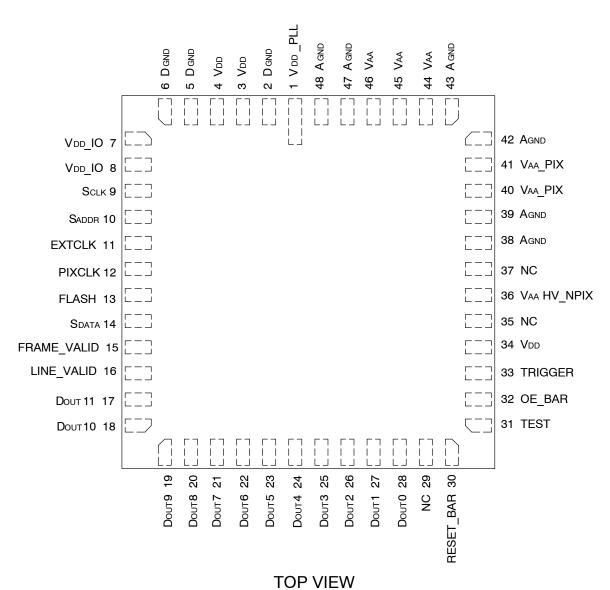
Figure 4. PLCC Pinout
