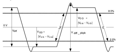
Figure 9. Single-Ended and Differential Signals
