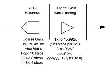
Figure 24. Gain Stages in AR0330CS Sensor
