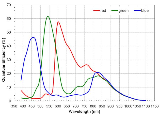
Figure 39. Bare Die Quantum Efficiency
