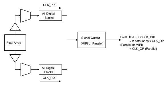
Figure 17. Sensor Dual Readout Paths
