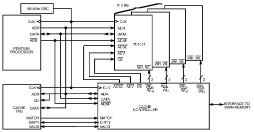
Figure 1. Cache Using Four CY7C1031s
