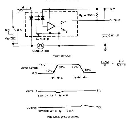
FIGURE 2. TRANSIENT IMMUNITY TEST CIRCUIT AND WAVEFORMS
