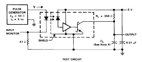
NOTE A:  $C_L$  is approximately 15 pF, which includes probe and stray wiring capacitances
