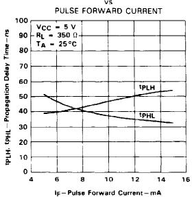
PROPAGATION DELAY TIME FROM LED INPUT vs
