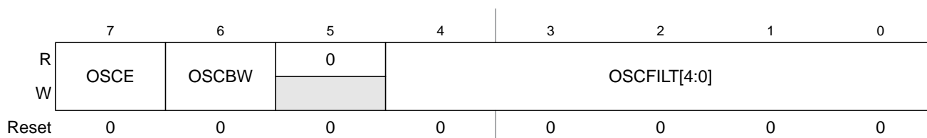
Figure 7-29. S12CPMU Oscillator Register (CPMUOSC)
