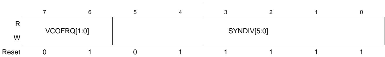
Figure 7-4. S12CPMU Synthesizer Register (CPMUSYNR)
