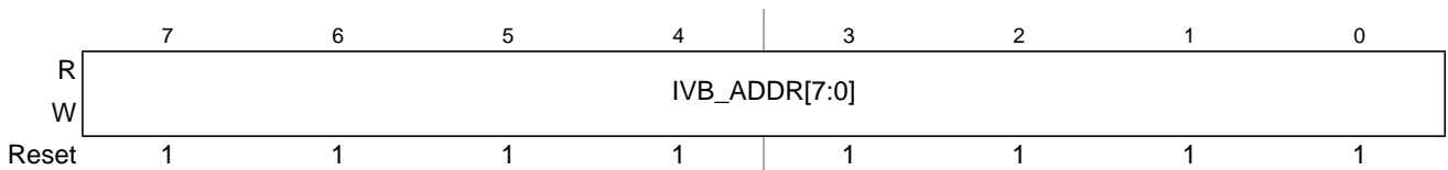
Figure 4-2. Interrupt Vector Base Register (IVBR)
