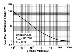
Figure 12. Single Pulse Maximum Power Dissipation
