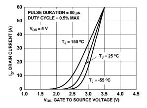
Figure 5. Transfer Characteristics
