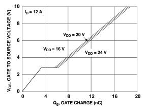
Figure 7. Gate Charge Characteristics
