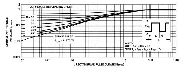
Figure 13. Junction-to-Ambient Transient Thermal Response Curve
