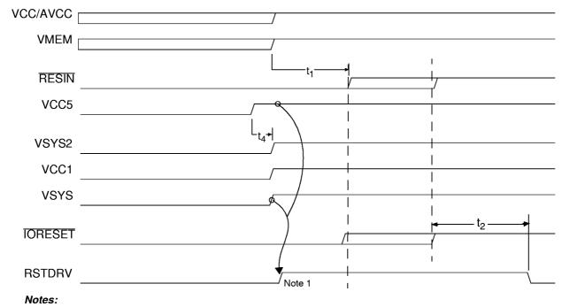
1. RSTDRV external driver is powered by: VCCIO = VSYS and VCC Clamp = VCC5.
