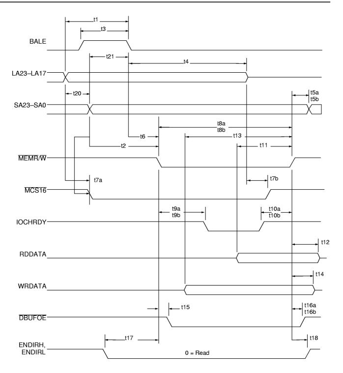
Figure 51. ISA Memory Read/Write 16-Bit Cycle
