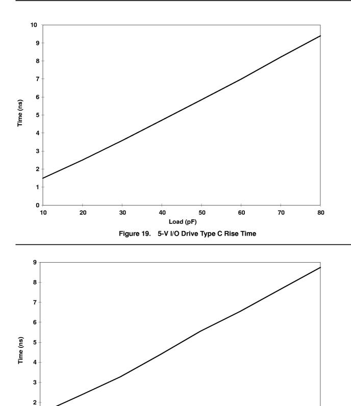
Load (pF) Figure 20. 5-V I/O Drive Type C Fall Time
