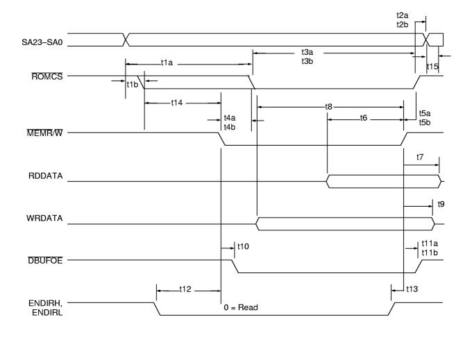
Figure 47. BIOS ROM Read/Write 8-Bit Cycle
