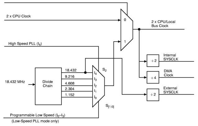
Figure 2. Clock Steering Block Diagram
