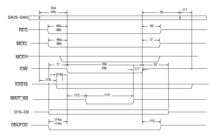
Figure 46. PCMCIA I/O Write Cycle
