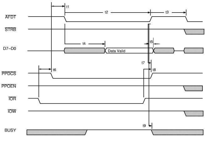
Figure 56. EPP Data Register Read Cycle
