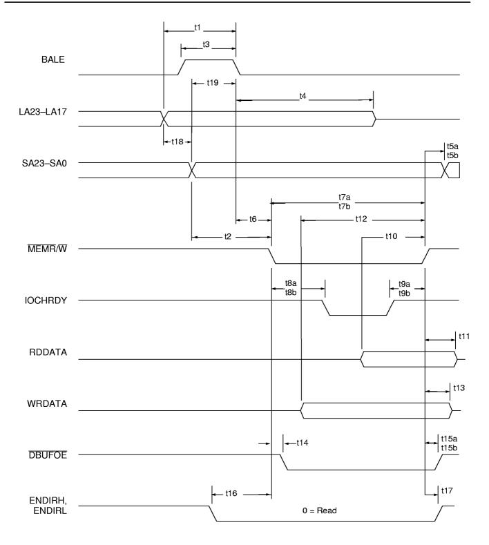
Figure 50. ISA Memory Read/Write 8-Bit Cycle
