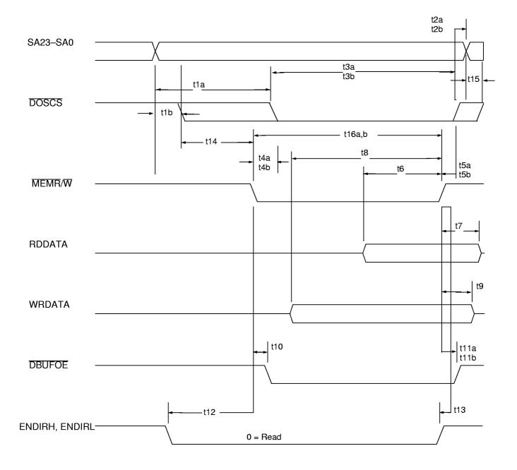
Figure 49. DOS ROM Read/Write 16-Bit Cycle
