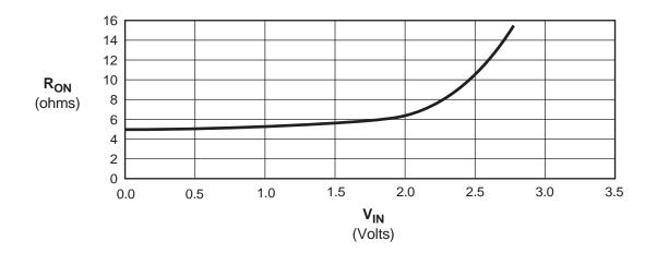
Note: For QS32253, add 23 $\Omega$  to  $R_{\text{ON}}$  shown.
