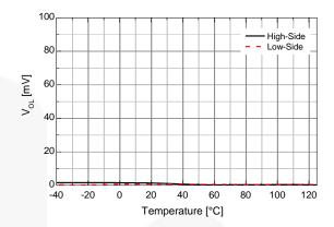
Figure 22.High-Level Output Voltage vs. Temperature
