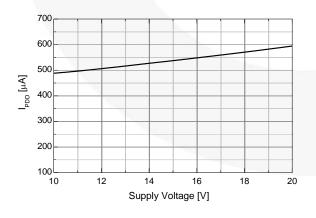
Figure 31. Quiescent V<sub>BS</sub> Supply Current vs. Supply Voltage
