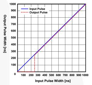
Figure 46. Input Filter Characteristic of Narrow ON
