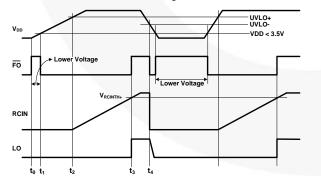
Figure 38. Waveforms for Under-Voltage Lockout
