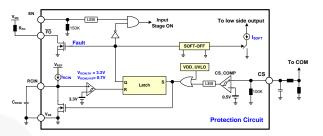
**Figure 42. Over-Current Protection**
