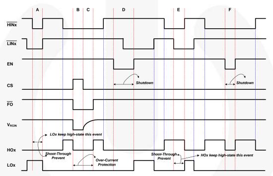
Figure 35. Input / Output Timing Diagram
