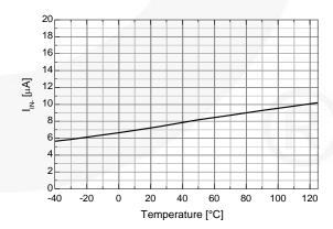
Figure 26.Logic Input HIGH Bias Current vs. Temperature
