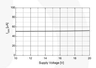
Figure 30. Quiescent V<sub>DD</sub> Supply Current vs. Supply Voltage
