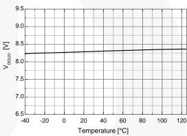
Figure 18. V<sub>DD</sub> UVLO+ vs. Temperature
