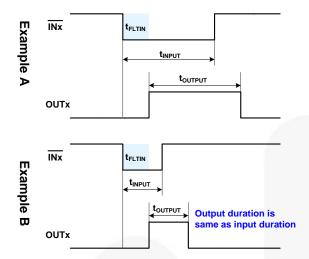
**Figure 44.Input Noise Filter Definition**
