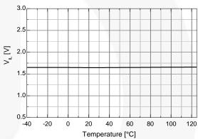
Figure 24.Logic HIGH Input Voltage vs. Temperature
