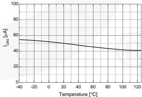
Figure 14. Quiescent V<sub>DD</sub> Supply Current vs. Temperature
