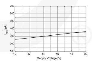
Figure 32. Operating V<sub>DD</sub> Supply Current vs. Supply Voltage
