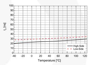
Figure 6. Turn-On Rise Time vs. Temperature
