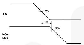
Figure 41. Output Enable Timing Waveform
