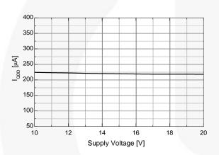
Figure 29. Enable Pin Pull-Down Resistance vs. Supply Voltage
