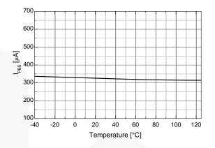
Figure 16. Operating V<sub>DD</sub> Supply Current vs. Temperature
