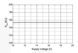
Figure 28. Input Pull-Down Resistance vs. Supply Voltage
