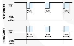
Figure 45. Noise Rejecting Input Filter Definition
