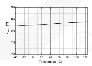
Figure 20.V<sub>BS</sub> UVLO+ vs. Temperature
