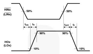
Figure 34. Switching Time Waveform Definitions
