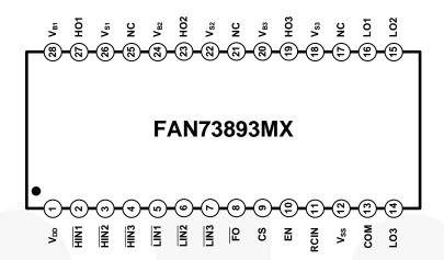
Figure 3. Pin Assignments
