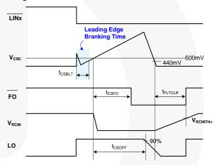
Figure 43. R<sub>CIN</sub> and Fault-Clear Waveform Definition
