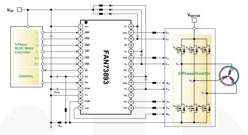
Figure 1. 3-Phase BLDC Motor Drive Application
