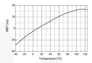
Figure 10. Dead Time vs. Temperature
