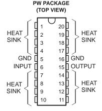
HEAT SINK – These pins have an internal resistive connection to ground and should be grounded or electrically isolated.
