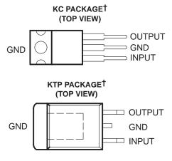
† The GND terminal is in electrical contact with the mounting base.
