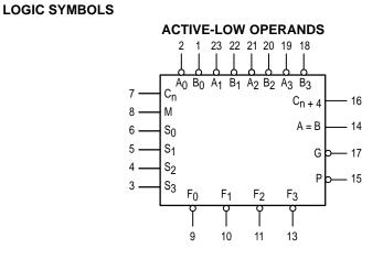
V<sub>CC</sub> = PIN 24 GND = PIN 12
