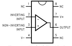
Figure 1. 8-Pin SOIC (Top View)
