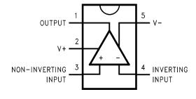
Figure 2. 5-Pin SOT-23 (Top View)
