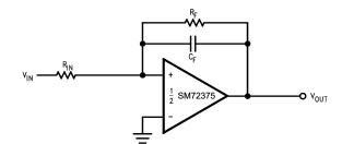
Figure 25. Canceling the Effect of Input Capacitance
