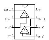
Figure 1. 8-Pin VSSOP - Top View Package Number DGK
