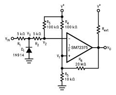
Figure 29. Zero Crossing Detector
