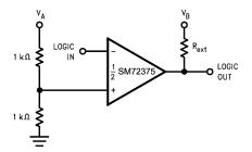
Figure 26. Universal Logic Level Shifter
