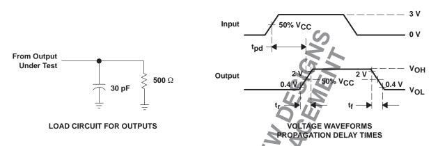
NOTES: A.  $C_L$  includes probe and jig capacitance.
