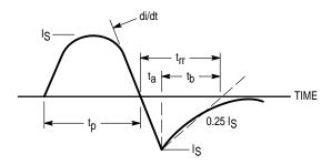
Figure 15. Diode Reverse Recovery Waveform
