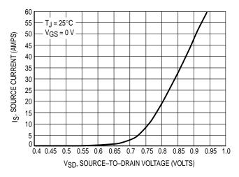
Figure 10. Diode Forward Voltage versus Current
