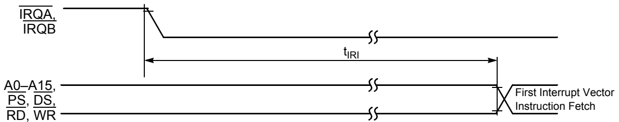
Figure 10-9 Interrupt from Wait State Timing
