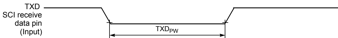
Figure 10-18 TXD Pulse Width
