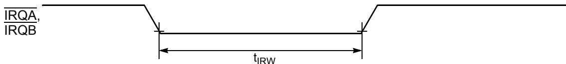
Figure 10-7 External Interrupt Timing (Negative Edge-Sensitive)
