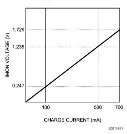
FIGURE 4. IMON Voltage vs Charge Current
