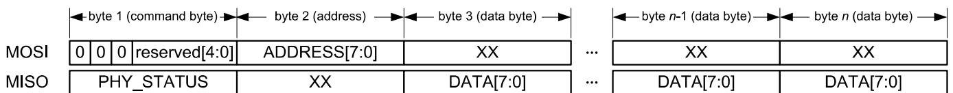
Figure 6-11. Packet Structure – SRAM Read Access.
