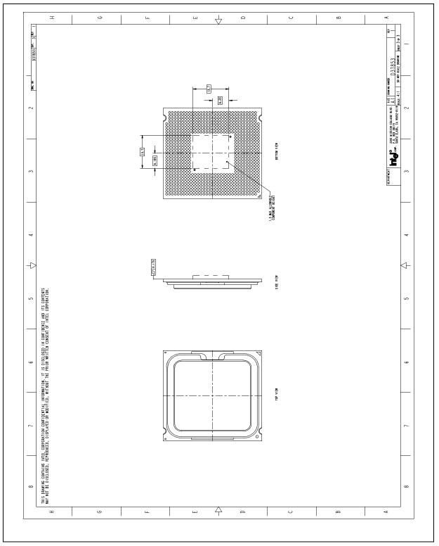
Figure 3-4. Processor Package Drawing (Sheet 3 of 3)
