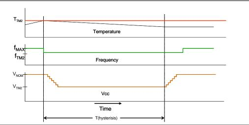
The PROCHOT# signal is asserted when a high temperature situation is detected, regardless of whether TM1 or TM2 is enabled.
