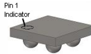
Figure 4. WLCSP Bumps Facing Down (Bottom View)
