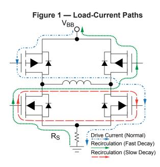
The user selects an external resistor  $(R_T)$  and capacitor  $(C_T)$  to determine the time period  $(t_{OFF} = R_T \times C_T)$  during which the drivers remain disabled (see RC Fixed Off-Time section, below). At the end of the RC interval, the drivers are enabled allowing the load current to increase again. The PWM cycle repeats, maintaining the peak load current at the desired value (figure 2).
