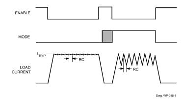
**Brake Operation.** During braking, care should be taken to ensure that the motor's current does not exceed the ratings of the device. The braking current can be measured by using an oscilloscope with a current probe connected to one of the motor's leads, or if the back-EMF voltage of the motor is known, approximated by:
