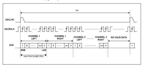
Figure 30 DSP Mode Audio Interface - Mode B Slave, DAC
