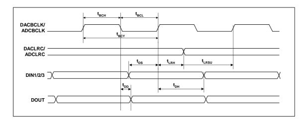
Figure 41 Digital Audio Data Timing - Slave Mode
