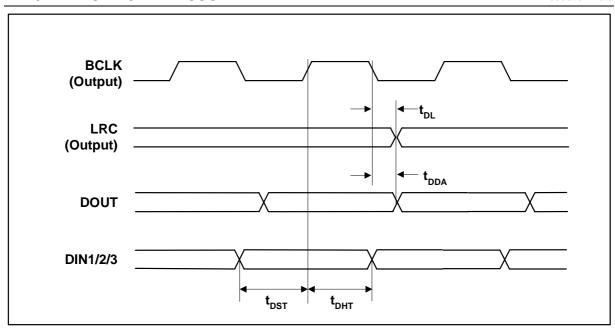
Figure 15 Digital Audio Data Timing – Master Mode
