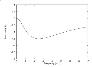
Figure 7 De-Emphasis Frequency Response (32kHz)
