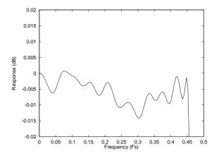
Figure 5 ADC Digital Filter Frequency Response
