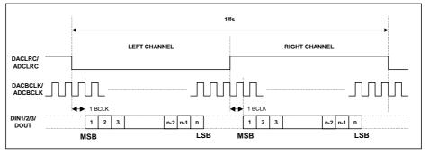
Figure 49 I<sup>2</sup>S Mode Timing Diagram
