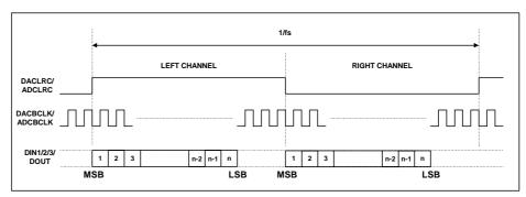
Figure 23 Left Justified Mode Timing Diagram
