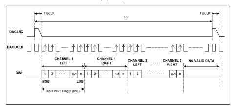
Figure 50 DSP Mode Audio Interface - Mode A Slave, DAC
