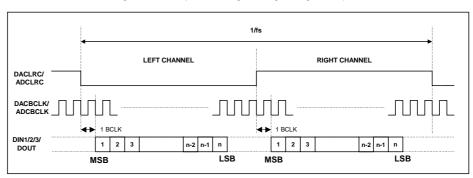
Figure 25 I<sup>2</sup>S Mode Timing Diagram
