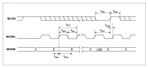
Figure 18 SPI Compatible Control Interface Input Timing
