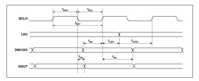
Figure 17 Digital Audio Data Timing - Slave Mode
