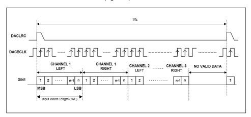
Figure 54 DSP Mode Audio Interface - Mode B Slave, DAC
