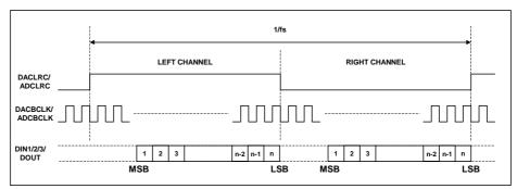
Figure 24 Right Justified Mode Timing Diagram
