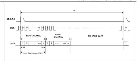
Figure 56 DSP Mode Audio Interface - Mode A Slave, ADC
