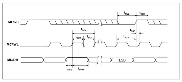
Figure 42 SPI Compatible Control Interface Input Timing
