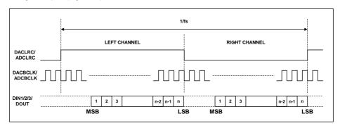
Figure 48 Right Justified Mode Timing Diagram
