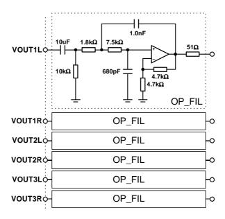
Figure 59 Recommended Post DAC Filter Circuit
