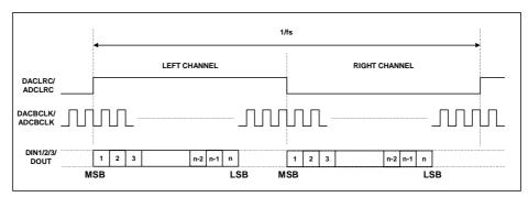
Figure 47 Left Justified Mode Timing Diagram
