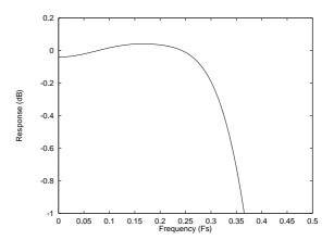
Figure 3 DAC Digital Filter Frequency Response
