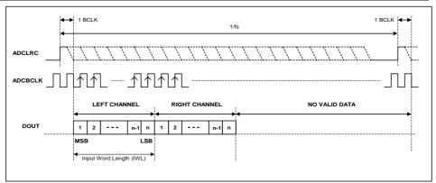
Figure 53 DSP Mode Audio Interface - Mode A Master, ADC
