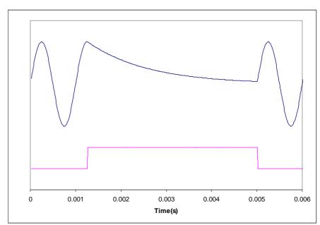
Figure 19 Application and Release of Soft Mute
