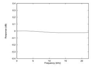
Figure 9 De-Emphasis Frequency Response (44.1KHz)
