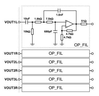
Figure 35 Recommended Post DAC Filter Circuit
