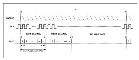
Figure 57 DSP Mode Audio Interface - Mode B Master, ADC
