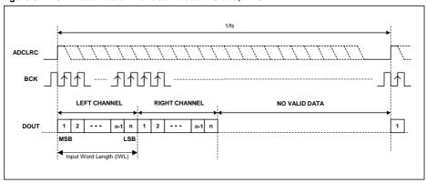
Figure 33 DSP Mode Audio Interface - Mode B Master, ADC
