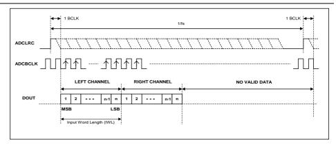
Figure 29 DSP Mode Audio Interface - Mode A Master, ADC
