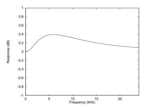
Figure 11 De-Emphasis Frequency Response (48kHz)
