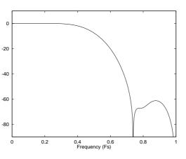
Figure 2 DAC Digital Filter Ripple -44.1, 48 and 96kHz
