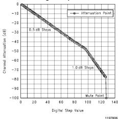
FIGURE 3. LM1972 Attenuation Step Scheme
