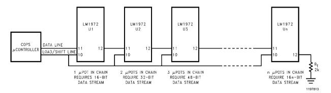
FIGURE 11. n-µPot Daisy-Chained Circuit
