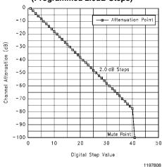
FIGURE 5. LM1972 2.0dB Attenuation Step Scheme
