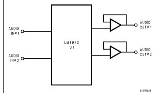
FIGURE 1. Typical Audio Attenuator Application Circuit
