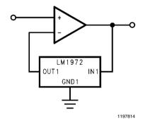
FIGURE 10. Digitally-Controlled Logarithmic Gain Amplifier Circuit
