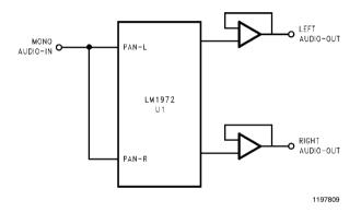
**FIGURE 6. Mono Panning Circuit**
