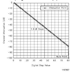
FIGURE 4. LM1972 1.0dB Attenuation Step Scheme
