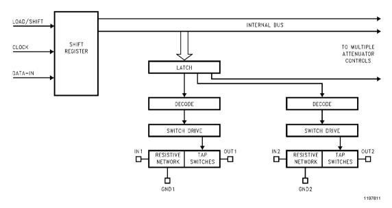
FIGURE 9. µPot System Architecture
