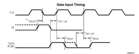
\*To reset these devices, CLK and  $\overline{CS}$  must be simultaneously high for a period of t<sub>SELECT</sub> or greater. Otherwise these devices are compatible with industry standards ADC0831/2/4/8.
