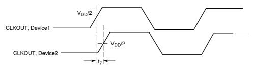
Figure 8. Device-Device Skew
