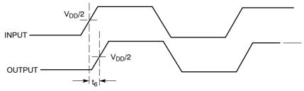
Figure 7. Input-Output Propagation Delay
