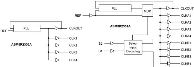
Figure 1. Block Diagram
