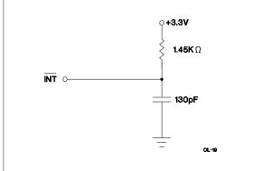
Figure 6. Output Load A—bq3285L
