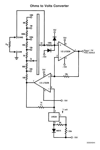
$$V_{O} = \frac{1V}{R_{LADDER}} \times R_{X}$$
