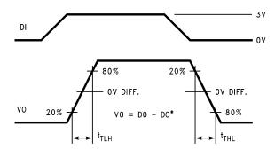
Figure 4. Driver Differential Transition Timing
