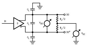
Figure 1.  $\,V_{\text{OD}}$  and  $\,V_{\text{OC}}$  Test Circuit
