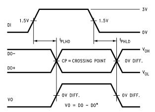
Figure 3. Driver Differential Propagation Delay Timing
