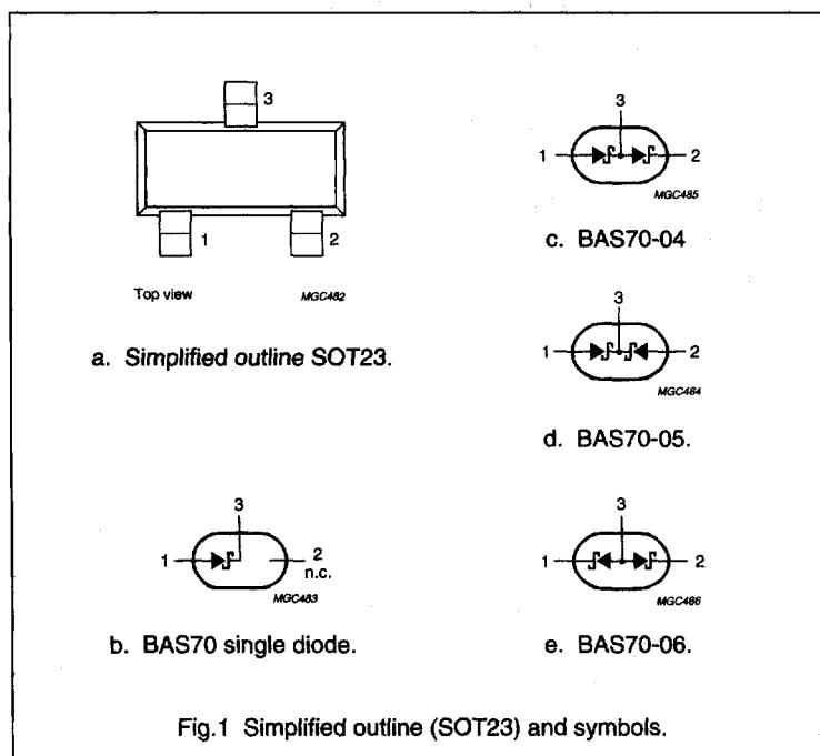
**Fig.1 Simplified outline (SOT23) and symbols.**
