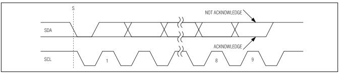
Figure 4. Acknowledge and Not-Acknowledge Bits
