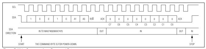
Figure 7. Write Sequence for a Command Byte
