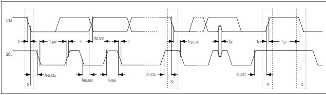
Figure 1. 2-Wire, Serial-Interface Timing Diagram
