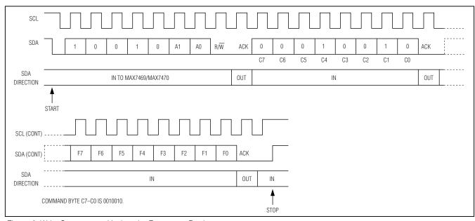
Figure 6. Write Sequence to Update the Frequency Register
