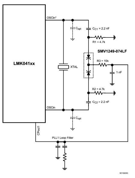
FIGURE 6. Reference Design Circuit for Crystal Oscillator Option
