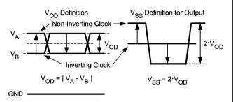
Two Different Definitions for Differential Output Signals
