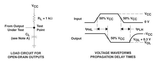
NOTES: A.  $C_{\mbox{L}}$  includes probe and jig capacitance.
