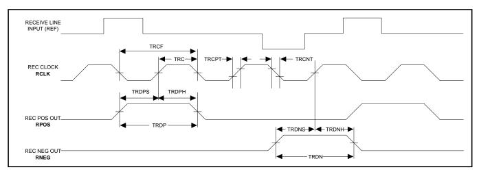
**FIGURE 2: Receive Waveforms**
