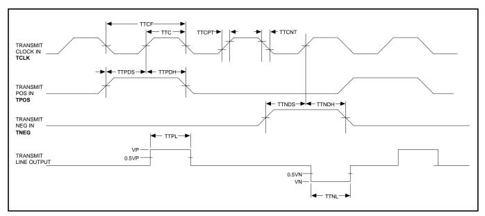
FIGURE 3: Transmit Waveforms
