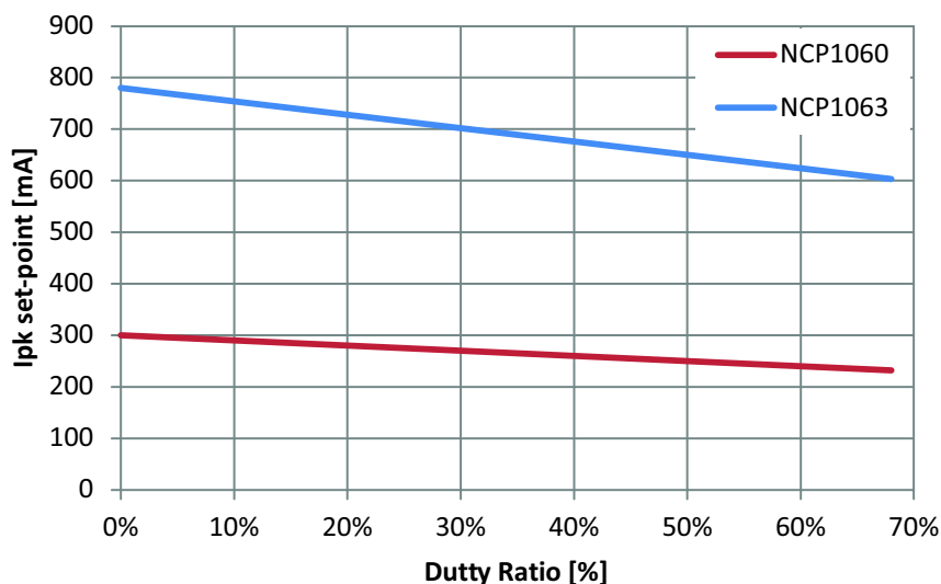
Figure 44. I pk Set-point Varies with Power Switch on Time, which is Caused by the Ramp Compensation
