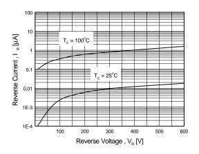
Figure 2. Typical Reverse Current vs. Reverse Voltage
