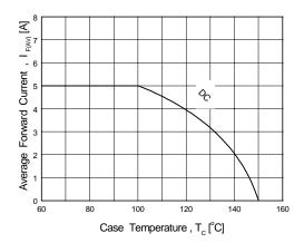
Figure 6. Forward Current Derating Curve
