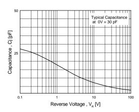
Figure 3. Typical Junction Capacitance
