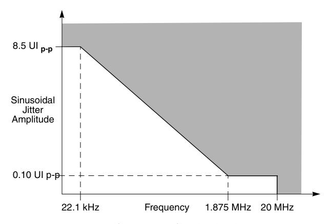
Figure 42. Single Frequency Sinusoidal Jitter Limits
