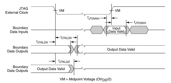
Figure 33. Boundary-Scan Timing Diagram
