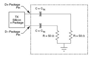
Figure 39. Compliance Test/Measurement Load
