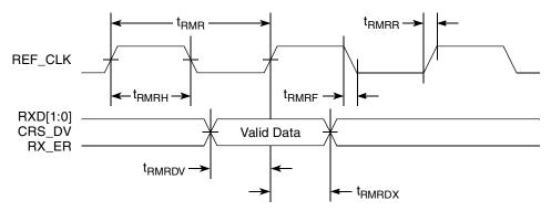
Figure 21. RMII Receive AC Timing Diagram
