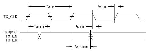
Figure 12. MII Transmit AC Timing Diagram
