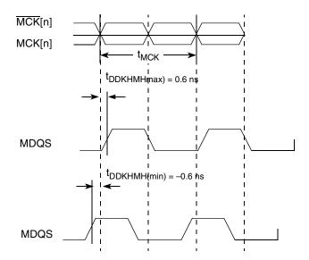
Figure 4. Timing Diagram for tDDKHMH
