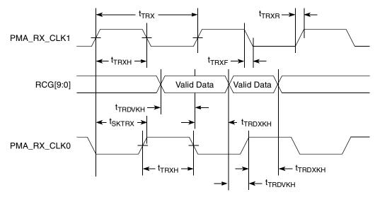
Figure 16. TBI Receive AC Timing Diagram
