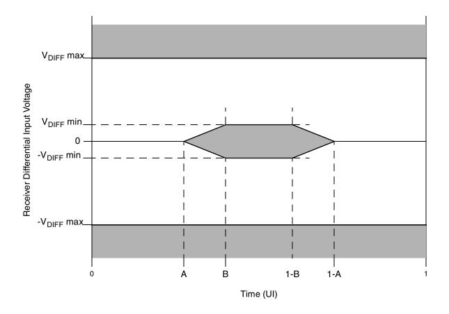
Figure 43. Receiver Input Compliance Mask
