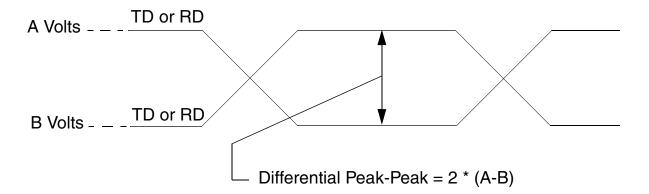
Figure 40. Differential Peak-Peak Voltage of Transmitter or Receiver
