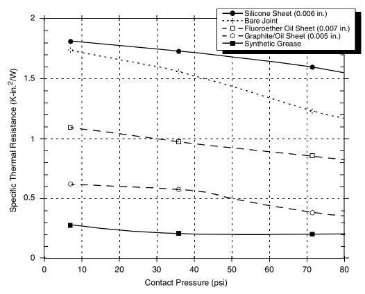
Figure 48. Thermal Performance of Select Thermal Interface Material
