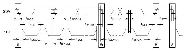
Figure 35. I<sup>2</sup>C Bus AC Timing Diagram
