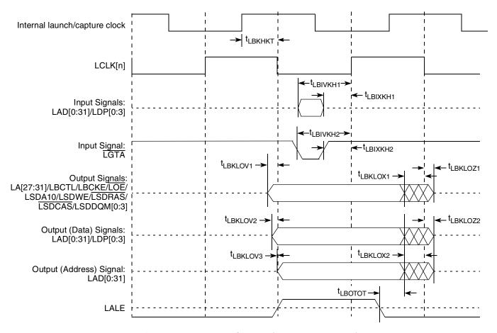
Figure 25. Local Bus Signals (PLL Bypass Mode)
