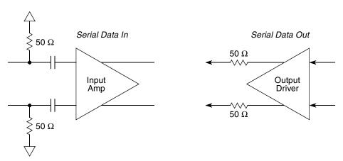
Figure 36. Driver and Receiver of SerDes (PCI Express, Serial RapidIO, and SD REF CLK/SD REF CLK
