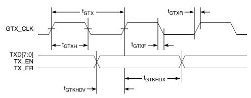
Figure 9. GMII Transmit AC Timing Diagram
