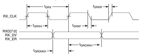
Figure 11. GMII Receive AC Timing Diagram
