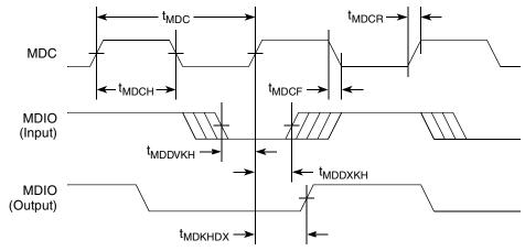
Figure 22. MII Management Interface Timing Diagram
