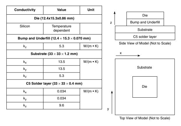
Figure 49. Recommended Thermal Model of MPC8641
