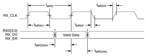
Figure 14. MII Receive AC Timing Diagram
