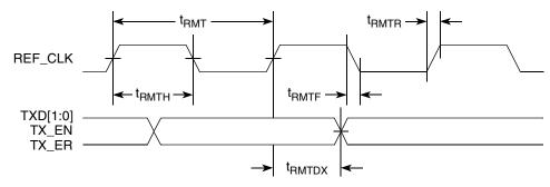
Figure 19. RMII Transmit AC Timing Diagram
