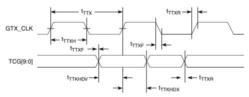
Figure 15. TBI Transmit AC Timing Diagram
