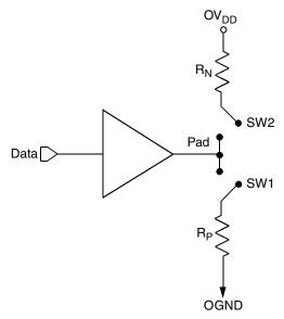
Figure 53. Driver Impedance Measurement
