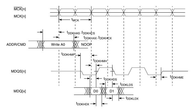
Figure 5. DDR SDRAM Output Timing Diagram
