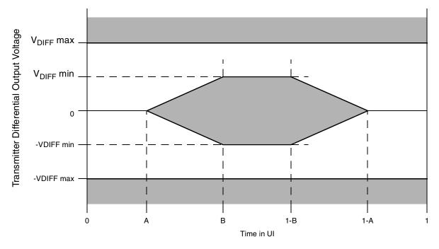
Figure 41. Transmitter Output Compliance Mask
