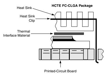
Figure 46. FC-CLGA Package Exploded Cross-Sectional View with Several Heat Sink Options
