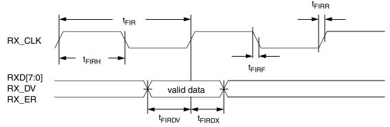
Figure 8. FIFO Receive AC Timing Diagram
