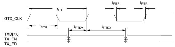
Figure 7. FIFO Transmit AC Timing Diagram
