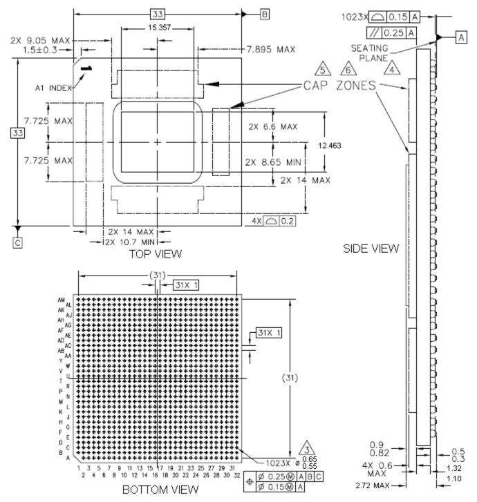
Figure 44. MPC8641 Lead-free or Eutetic Lead FC-CBGA Dimensions
