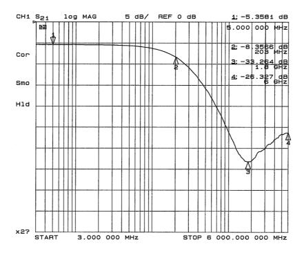
Figure 6. Insertion Loss vs. Frequency (FILTER5 Input to GND)
