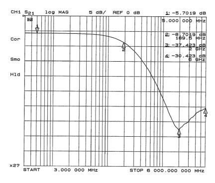
Figure 9. Insertion Loss vs. Frequency (FILTER8 Input to GND)
