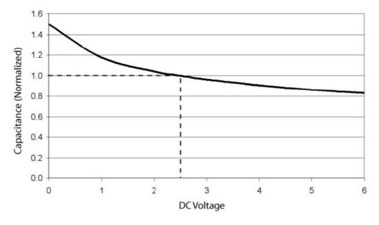
Figure 1. Filter Capacitance vs. Input Voltage (normalized to capacitance at 2.5 VDC and 25°C)
