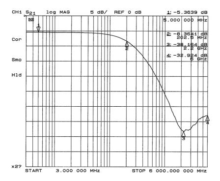
Figure 8. Insertion Loss vs. Frequency (FILTER7 Input to GND)
