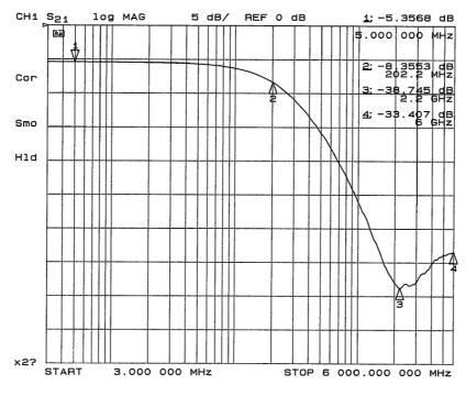
Figure 3. Insertion Loss vs. Frequency (FILTER2 Input to GND)
