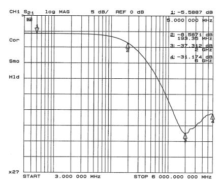
Figure 2. Insertion Loss vs. Frequency (FILTER1 Input to GND)
