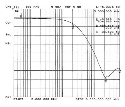
Figure 7. Insertion Loss vs. Frequency (FILTER6 Input to GND)
