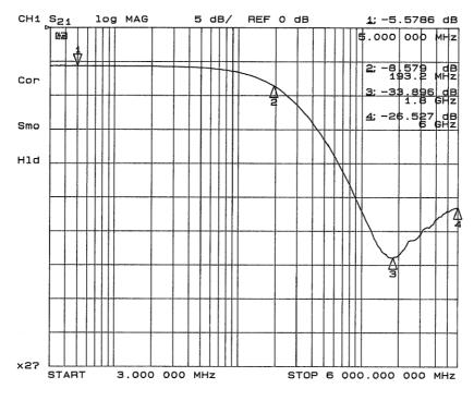
Figure 5. Insertion Loss vs. Frequency (FILTER4 Input to GND)
