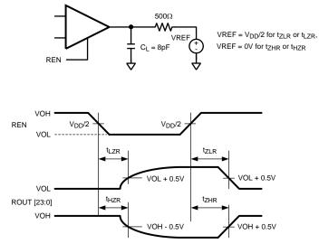
Note: CL includes instrumentation and fixture capacitance within 6 cm of ROUT[23:0]
