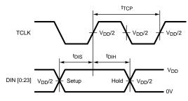
Figure 5. Serializer Setup/Hold Times
