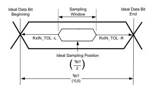
RxIN\_TOL\_L is the ideal noise margin on the left of the figure, with respect to ideal. RxIN\_TOL\_R is the ideal noise margin on the right of the figure, with respect to ideal.
