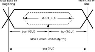
Figure 9. Transmitter Output Eye Opening (TxOUT\_E\_O)
