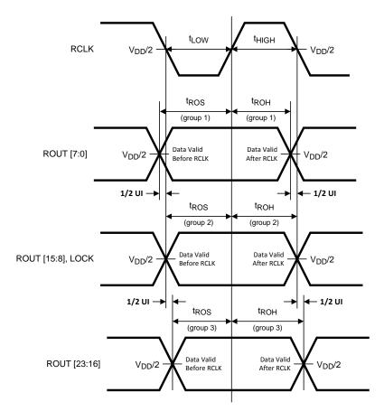
Figure 15. Deserializer Setup and Hold Times
