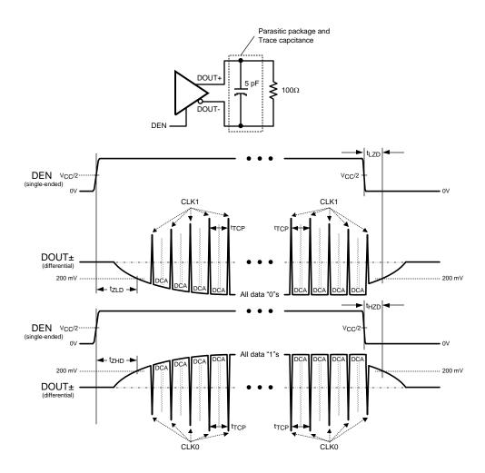
Figure 6. Serializer TRI-STATE Test Circuit and Delay
