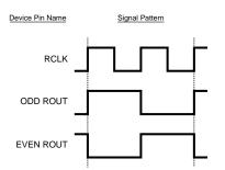
Figure 2. Deserializer Output Checker-board Pattern
