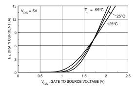
Figure 5. Transfer Characteristics.
