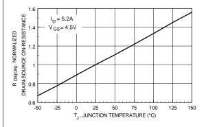
Figure 3. On-Resistance Variation with Temperature.
