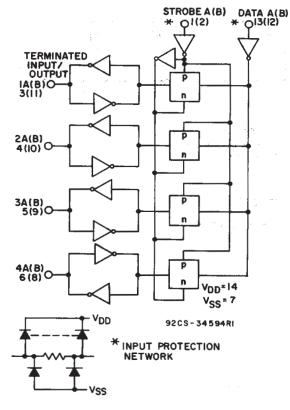
Fig. 1 - Logic diagram (½ of CD40117B)
