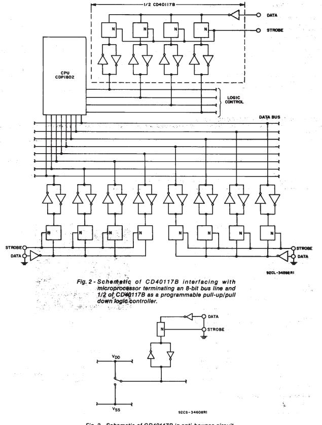
Fig. 3 - Schematic of CD40117B in anti-bounce circuit application.
