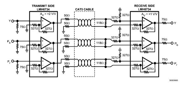
FIGURE 11. Component Video Transmission Over UTP (CAT5)
