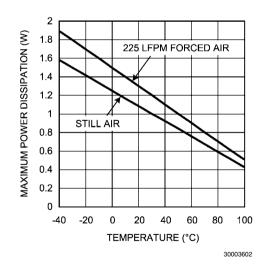
FIGURE 14. Maximum Power Dissipation
