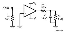
FIGURE 13. Decoupling Capacitive Loads
