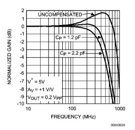
FIGURE 8. Frequency Response for Circuit in Figure 7
