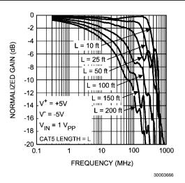
FIGURE 12. Frequency Response vs. Normalized Gain and CAT5 Cable Length
