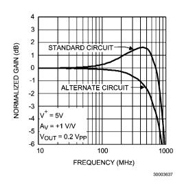
FIGURE 10. Frequency Response for Circuit in Figure 9 (Standard Circuit Figure 5)
