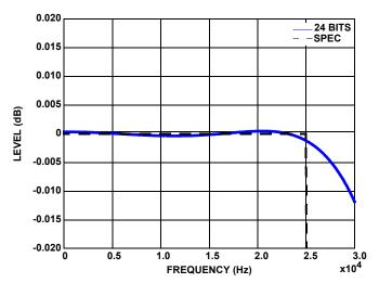
FIGURE 6. ADC DECIMATOR FREQUENCY RESPONSE (256 TAPS DECIMATE BY 32)
