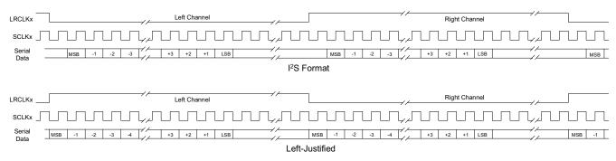
FIGURE 5. SAI PORT SUPPORTED DATA FORMATS FOR DELIVERY OF LINEAR PCM OR COMPRESSED AUDIO DATA
