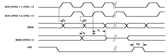
FIGURE 3. SPI TIMING
