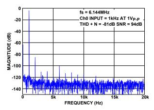
FIGURE 7. ADC PERFORMANCE AT FULL SCALE INPUT
