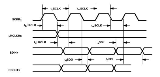
FIGURE 1. SERIAL AUDIO INTERFACE PORT TIMING
