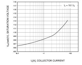
Figure 2. Base-Emitter Saturation Voltage
