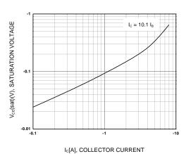
Figure 3. Collector-Emitter Saturation Voltage
