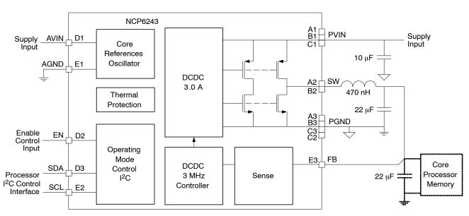
Figure 45. Typical Application Schematic
