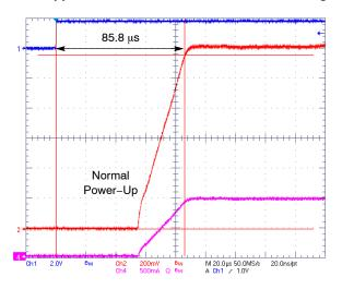
Figure 26. Normal Power Up, V<sub>OUT</sub> = 1.225 V
