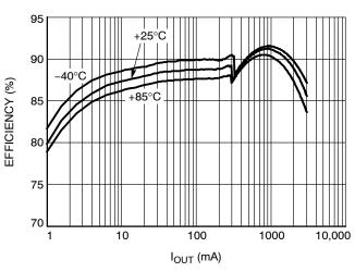
Figure 6. Efficiency vs.  $I_{LOAD}$  and  $V_{IN}$ V<sub>OUT</sub> = 1.225 V, SPM6530 Inductor
