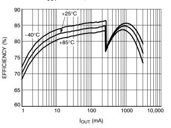
Figure 8. Efficiency vs.  $I_{LOAD}$  and  $V_{IN}$ V<sub>OUT</sub> = 0.60 V, SPM6530 Inductor
