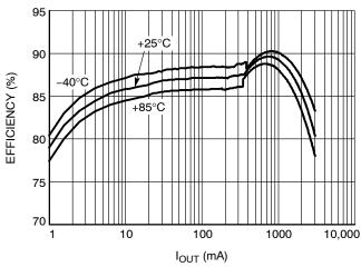
Figure 10. Efficiency vs.  $I_{\mbox{\scriptsize LOAD}}$  and  $V_{\mbox{\scriptsize IN}}$ V<sub>OUT</sub> = 1.225 V, PIFE20161B Inductor
