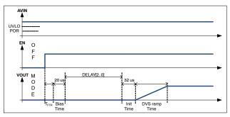
Figure 34. Normal Power Up Sequence (EN pin)
