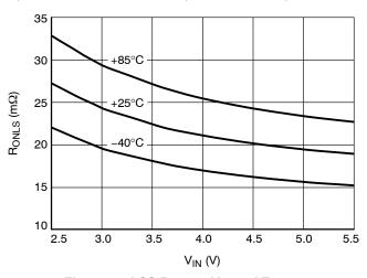
Figure 16. HSS R<sub>ON</sub> vs. V<sub>IN</sub> and Temperature
