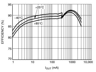
Figure 4. Efficiency vs. I<sub>LOAD</sub> and V<sub>IN</sub> V<sub>OUT</sub> = 1.39375 V, SPM6530 Inductor
