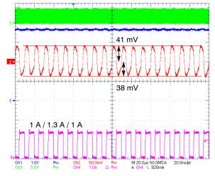
Figure 31. Fast Transient Load 0.1 - 1.4 A Auto Mode
