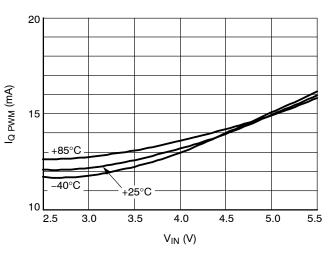
Figure 20.  $I_{\mbox{\scriptsize Q PFM}}$  vs.  $V_{\mbox{\scriptsize IN}}$  and Temperature
