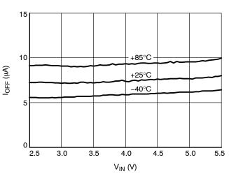
Figure 18.  $I_{OFF}$  vs.  $V_{IN}$  and Temperature
