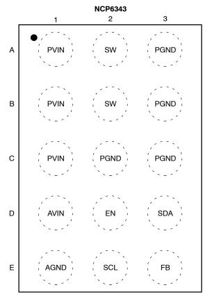
Figure 3. Pin Out (Top View)
