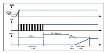
Figure 33. Initial Power Up Sequence
