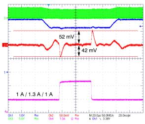
Figure 29. Transient Load 1.0 - 2.3 A Transient Line 4.2 - 3.6 V Auto Mode
