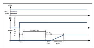
Figure 35. Quick Power Up Sequence (EN pin)
