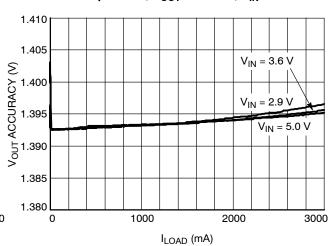
Figure 14.  $V_{OUT}$  Accuracy vs.  $I_{LOAD}$  and  $V_{IN}$   $V_{OUT}$  = 0.60 V
