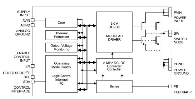
Figure 2. Simplified Block Diagram
