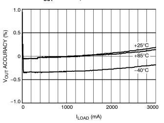
Figure 12.  $V_{OUT}$  Accuracy vs.  $I_{LOAD}$  and  $V_{IN}$   $V_{OUT}$  = 1.225 V
