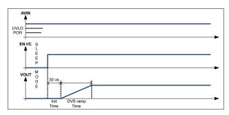
Figure 36. Fast Power Up Sequence (EN bit)
