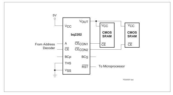
Figure 1. Hardware Hookup (5% Supply Operation)
