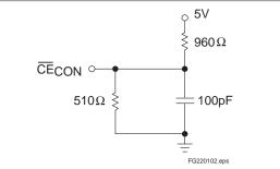
Figure 3. Output Load
