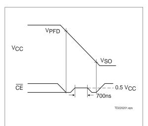
Figure 2. Battery Isolation Signal
