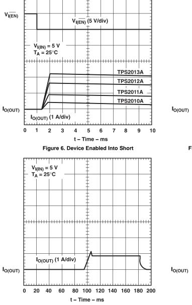
Figure 8. TPS2011A, Ramped Load on Enabled Device
