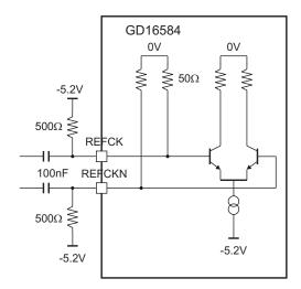
Figure 6. Reference Clock Input (REFCK/REFCKN), Differential AC Coupled.
