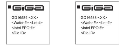
Figure 12. Device marking. Top view. The black square marks location of ball A1.
