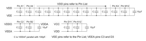
Figure 2. De-coupling of the Power Supply.
