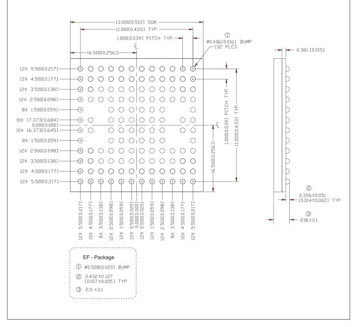
Figure 10. Package 132 ball ceramic BGA (EB and EF package). All dimensions are in mm.
