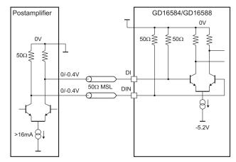
Figure 3. 10 Gbit/s Input (DI/DIN), DC Coupled
