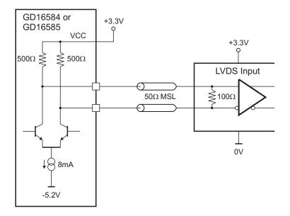
*Figure 5.* LVDS Compatible Output.
