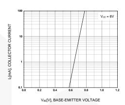
Figure 2. Transfer Characteristic
