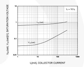
Figure 4. Base-Emitter Saturation Voltage and Collector-Emitter Saturation Voltage
