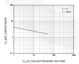
Figure 5. Output Capacitance
