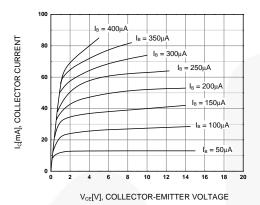
Figure 1. Static Characteristic
