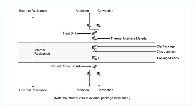
Heat generated on the active side of the chip is conducted through the silicon, then through the heat sink attach material (or thermal interface material), and finally to the heat sink; where it is removed by forced-air convection. Because the silicon thermal resistance is quite small, for a first-order analysis, the temperature drop in the silicon can be neglected. Thus, the heat sink attach material and the heat sink conduction/convective thermal resistances are the dominant terms.
