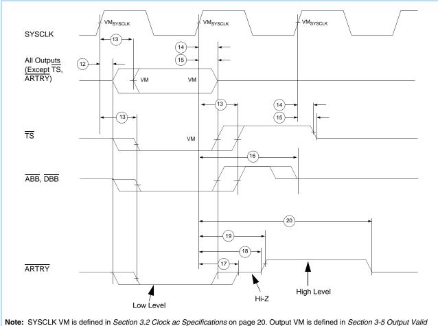
Figure 3-6. Output Timing Diagram for PowerPC 750FL RISC Microprocessor
