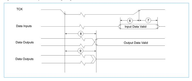
Figure 3-10. Test Access Port Timing Diagram
