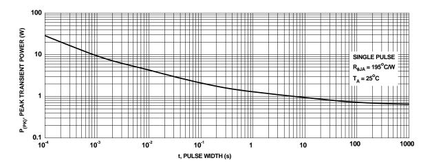
Figure 13. Single Pulse Maximum Power Dissipation
