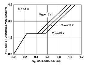
Figure 7. Gate Charge Characteristics
