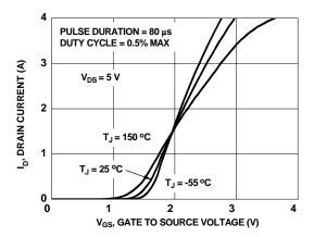
Figure 5. Transfer Characteristics
