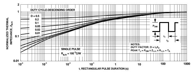
Figure 14. Junction-to-Ambient Transient Thermal Response Curve
