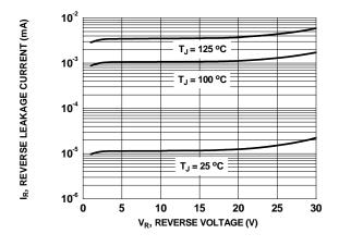
Figure 11. Schottky Diode Reverse Current
